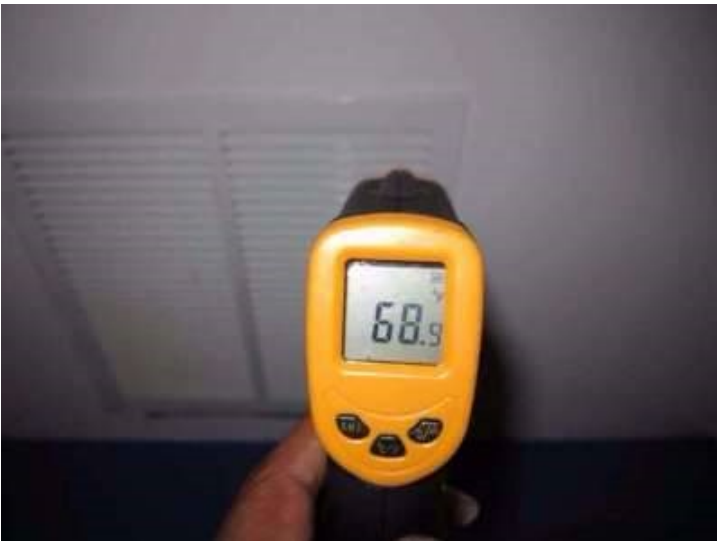
Photo 33-7 A/C Return 17 degree different Appeared serviceable
